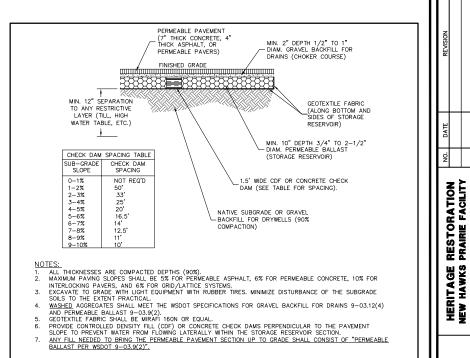
PERMEABLE PAVEMENT (BMP T5.15) SECTION
