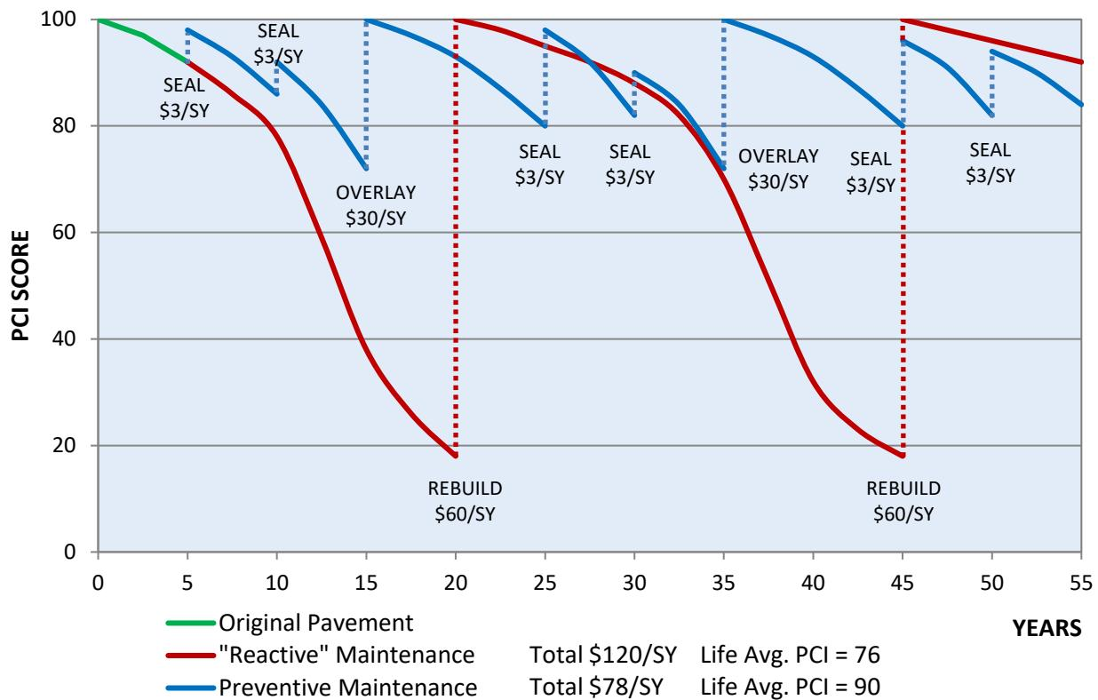
In the chart above, the red descending curves represent the “reactive” model of pavement treatment, in which roads deteriorate unchecked until they trigger major road rehabilitation. The blue curves illustrate the concept of pavement preservation, in which roads receive preventive maintenance regularly while still in good condition. Although prices for road treatments fluctuate and increase over time, the example serves to illustrate the obvious advantages to applying preventive maintenance.
